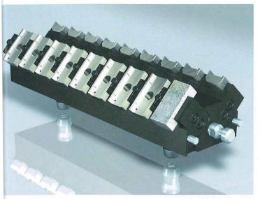
2 Special-purpose fixture for clamping a maximum of 18 components using the universal clamping system microClamp on an automatically exchangeable pallet (Photo: Triag International AG)
