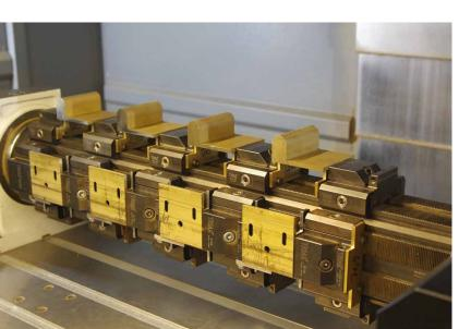
Tooling times minimised: thanks to the compact structure of the clamping modules, several components of the door fittings can be completely machined in a single process on the front and rear side on the clamping bridge.
