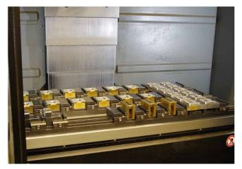
Productive thanks to multiple clamping: following a short tooling procedure, a large number of individual parts for glass door fittings can be manufactured without an operator. Photo: Konrad Mückel/MachPR
